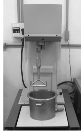
Fig. 2 – Partial view of the planetary rheometer.
