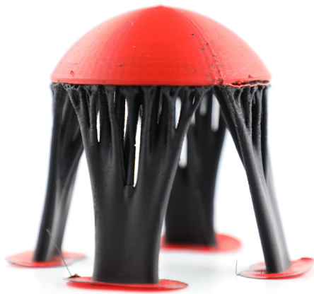
Fig. 17. 3D printed optimized supports for a tall dome (printed in an Ultimaker 3).
