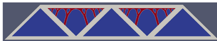
(a) Optimized support for MBB beam.
