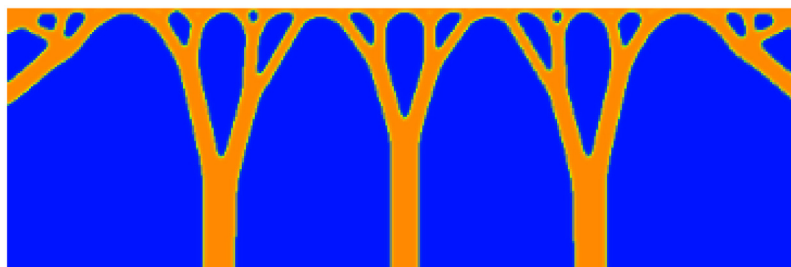
Fig. 8. Optimized self-supporting structure in a 3 \times 1 rectangular domain with 0-displacement boundary conditions on the bottom and on the sides of the domain.
