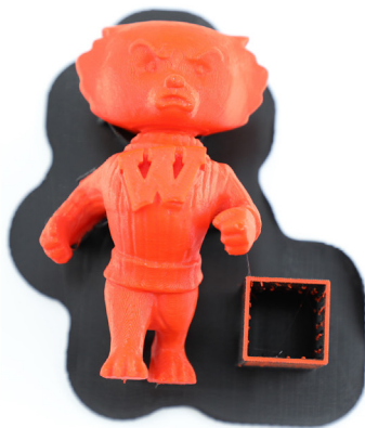
(c) Top view of 3D printed part with optimized supports
