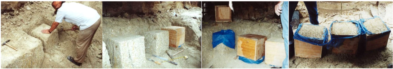
Fig. 2 Illustration of block sampling stages in residual soils the work at experimental site ES1 in Porto (adapted from [21])
