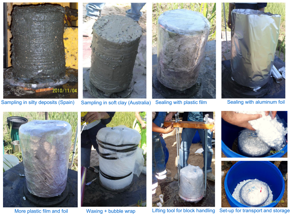
Fig. 26 Sherbrooke sampling campaigns in silty deposits (Spain) and soft clay (Australia)
