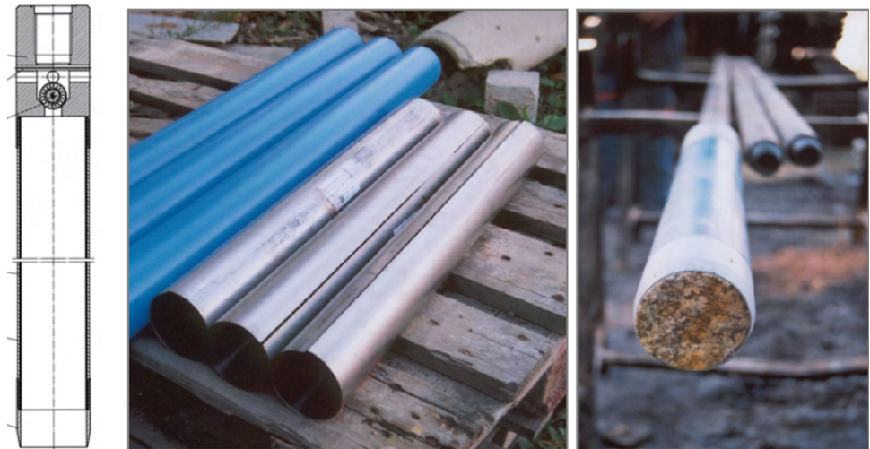
Fig. 4 NT 81 sampler: a schematic diagram; b photographs of the steel liner and of the sampler during sampling stage at the CICCOPN experimental site
