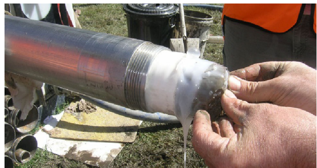
Fig. 9 Lubricating polymer gel coating soil sample (from [66])
