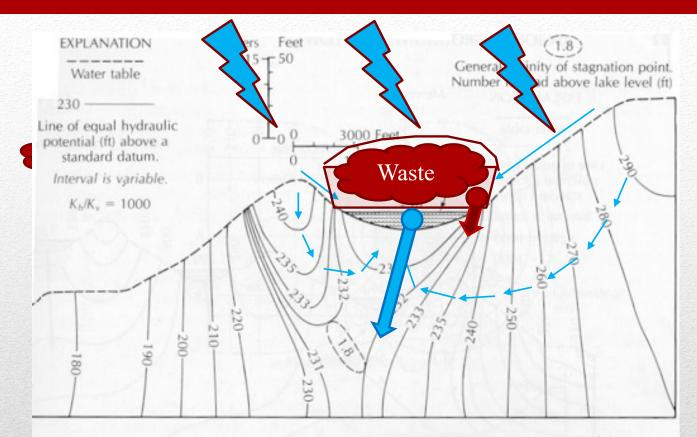
**FIGURE 8.26** Hydrogeologic cross section showing head distribution in a one-lake system with a homogeneous, anisotropic aquifer system. Results are based on a two-dimensional, steady-state, numerical-simulation model. Source: T. C. Winter, U.S. Geological Survey Professional Paper 1001, 1976.
