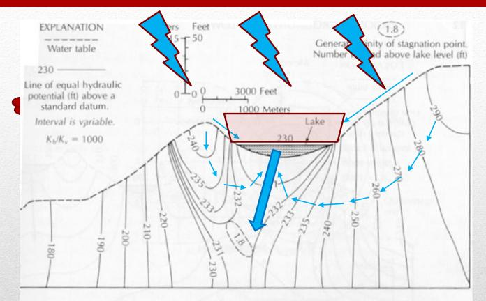
**FIGURE 8.26** Hydrogeologic cross section showing head distribution in a one-lake system with a homogeneous, anisotropic aquifer system. Results are based on a two-dimensional, steady-state, numerical-simulation model. Source: T. C. Winter, U.S. Geological Survey Professional Paper 1001, 1976.
