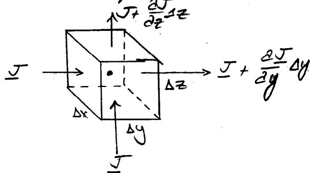
$$\partial = \frac{\partial}{\partial t} \int_{CV} C dV + \int_{CS} \underline{J} \cdot d\underline{A}$$
