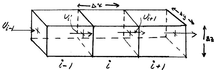
In cell balance models, the equivalent to Reynolds Transport Theorem is a material balance
