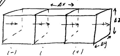
Mass in cell  $c_i \Delta x \Delta y \Delta z$ ; Rate of change of mass in cell  $\frac{\Delta c_i}{\Delta t} \Delta x \Delta y \Delta z$
