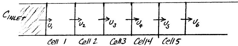
$$C_1^{t+\Delta t} = C_1^t + \frac{\Delta t}{\Delta x} (C_{\text{INLET}} U_1 - C_1^t U_2)$$
