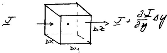
$$0 = \frac{\partial}{\partial t} \int_{CV} c dt + \int_{C.S.} c (\underline{V} \cdot d\underline{A})$$
