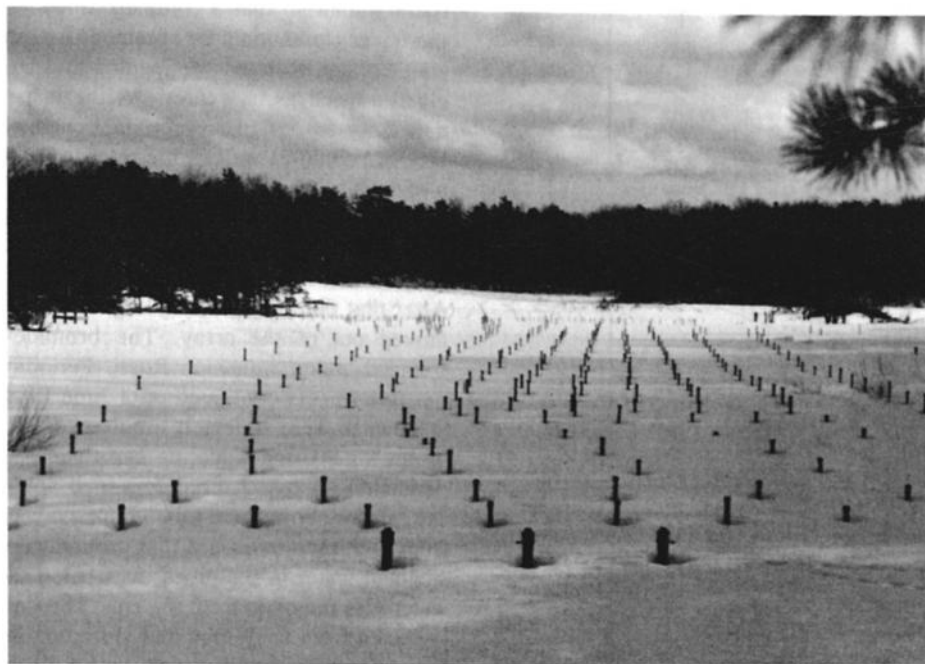
Fig. 7. View looking south of multilevel sampler array. The three injection wells are in foreground. Distance to trees is about 225 m. Photograph taken in February 1987.
