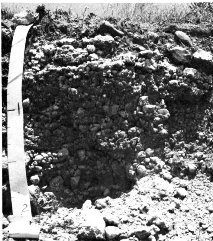
Figure 6.—Profile of a Polar soil showing many rounded and egg-shaped quartzite pebbles.
