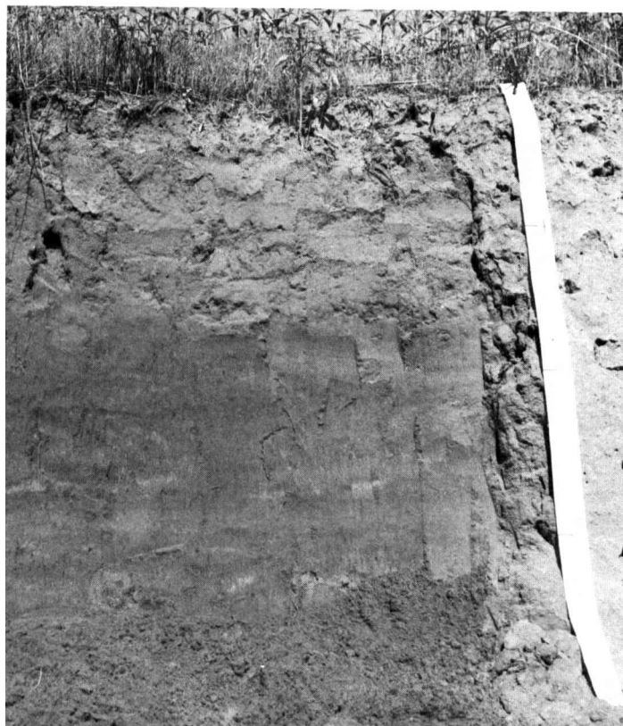
Figure 9.—Profile of a Springer loamy fine sand showing faintly expressed horizons. The upper 16 inches is loamy sand, and the underlying material is fine sandy loam.
