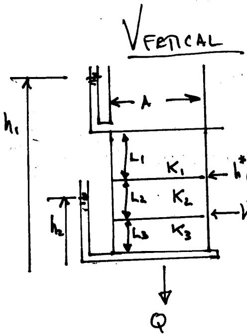
$$Q = \bar{K} A \frac{h_1 - h_2}{L_1 + L_2 + L_3} \therefore h_1 - h_2 = Q \frac{(L_1 + L_2 + L_3)}{\bar{K} A}$$
