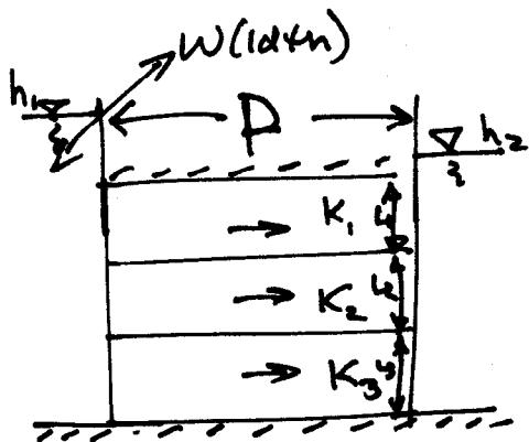
$$Q = \bar{K} A \frac{h_1 - h_2}{D} = \bar{K} (L_1 + L_2 + L_3) W \frac{h_1 - h_2}{D}$$
