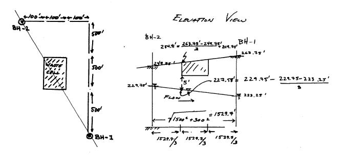
a) What is the hydraulic gradient, direction of groundwater flow, and average linear velocity of the groundwater (from the information given)?
