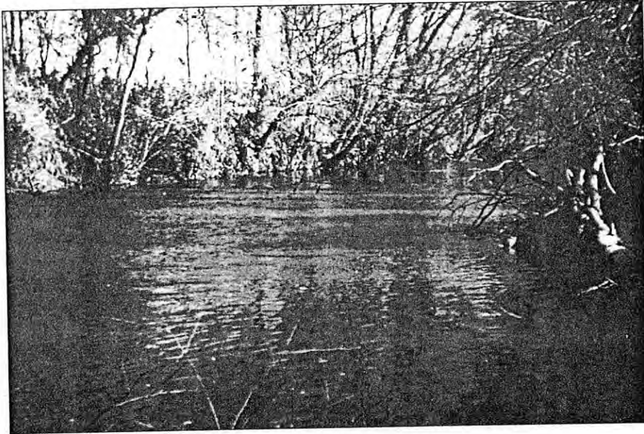
FIGURE 4.24 Etowah River near Dawsonville, Georgia: n = 0.041, 0.039, 0.035 ; depth = 9.8, 9.0, 4.4 ft. Bed is sand and gravel with several fallen trees in the reach. ( U.S. Geological Survey )
