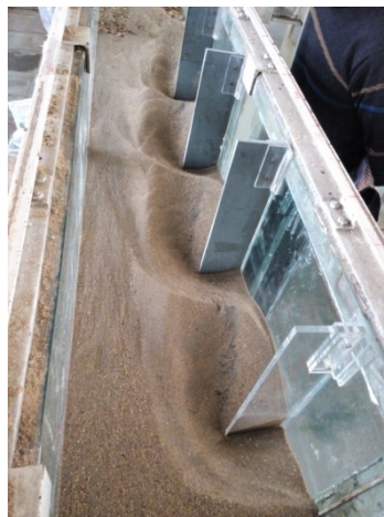
Fig. 8 The scour patterns of different flow rate with spur dikes spacing 4l
