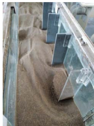
Fig. 6 The scour patterns of different flow rate with spur dikes spacing 3l
