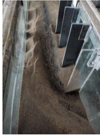
Fig. 4 The scour patterns of different flow rate with spur dikes spacing 2l
