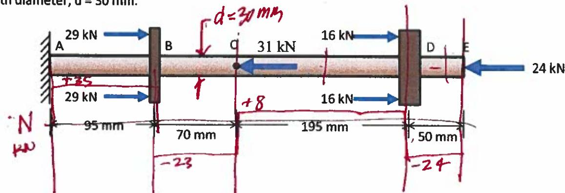
11) Calculate the axial normal stress in section BC, (6 pts)
