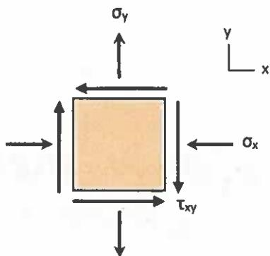
$$\begin{aligned}\sigma'_x &= -\frac{140+70}{2} + -\frac{140-70}{2}\cos 2(-30) + (-30)\sin 2(-30) \\ &= (-35) + (-52.5) + (25.98) \\ &= \boxed{-61.52 \text{ MPa (C)}}\end{aligned}$$
