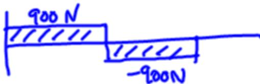
$$\begin{aligned}\tau &= \frac{3}{2} \frac{V}{bh} \\ &= \frac{3}{2} \frac{900N}{(0.02m)(0.06m)} \\ &= 1.125 \cdot 10^6 N/m^2 \\ &= 1.125 MPa\end{aligned}$$
