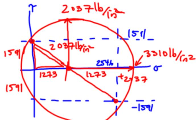
$$\begin{aligned}\sigma_x &= \frac{My}{I} \\ &= \frac{(2000 \text{ lb.in})(1\text{in})}{\frac{\pi(1\text{in})^4}{4}} \\ &= \frac{4(2000)(1)}{\pi} \\ &= 2546 \frac{\text{lb}}{\text{in}^2}\end{aligned}$$
