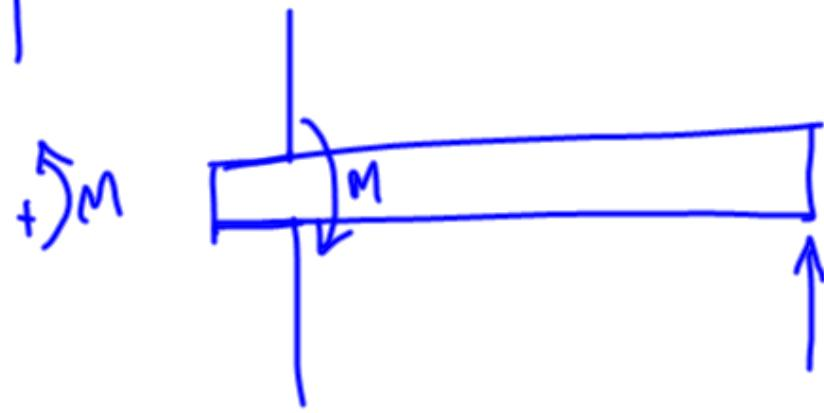
107. What is the maximum shearing stress at the fixed end of the 2 in. diameter shaft?
