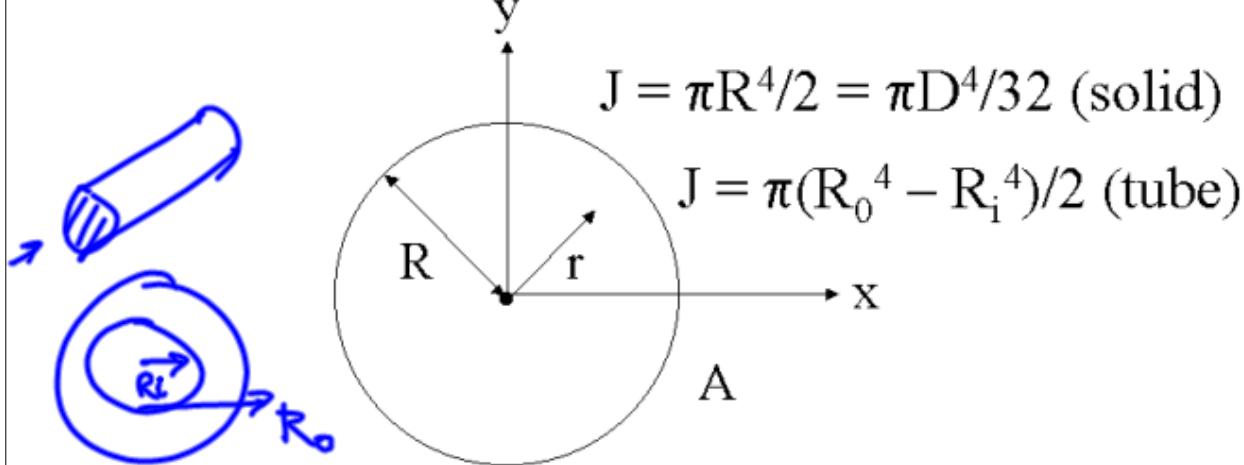
10.16 A 10 cm diameter shaft can tolerate up to a 140 MPa shear stress. What is the maximum torque (N·m)?
