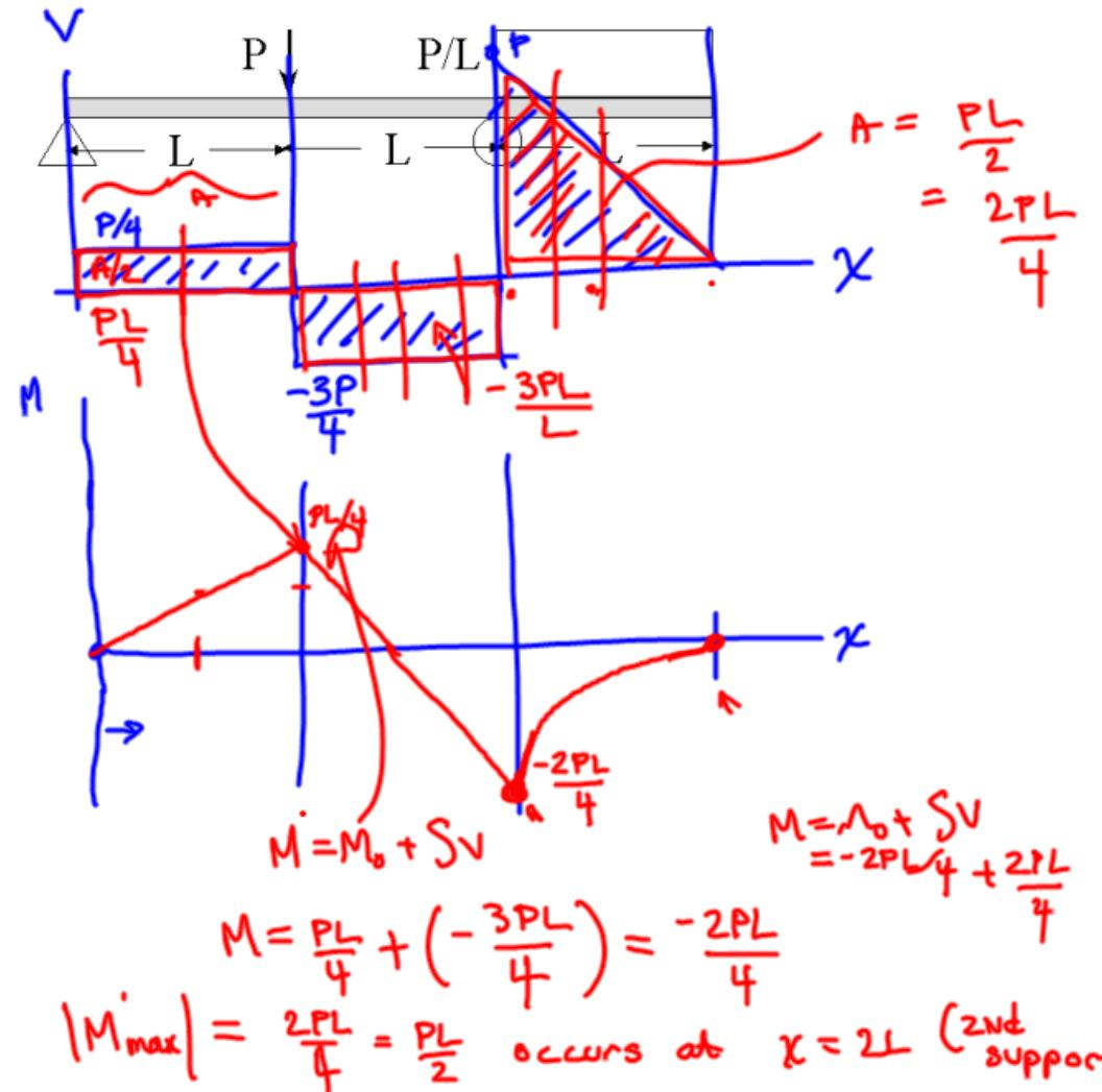
37. Sketch the shear and bending moment diagrams.
