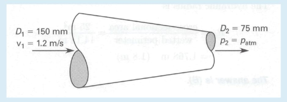
The gage pressure at the inlet is most nearly
