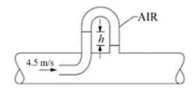
The reading h (m) on the manometer is most nearly:
