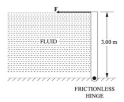
If the fluid on the left side of the gate has a density of  $1,750 \text{ kg/m}^3$ , the magnitude of the force **F** (kN) required to keep the gate closed is most nearly:
