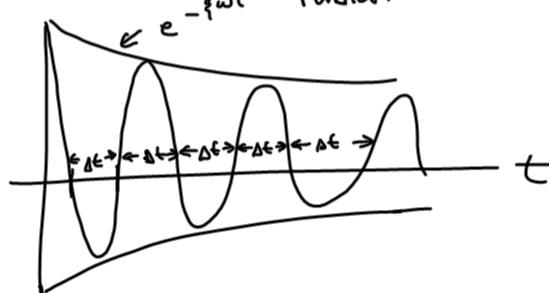
8. Find the damping ratio and natural frequency of a system described by the following equation.
