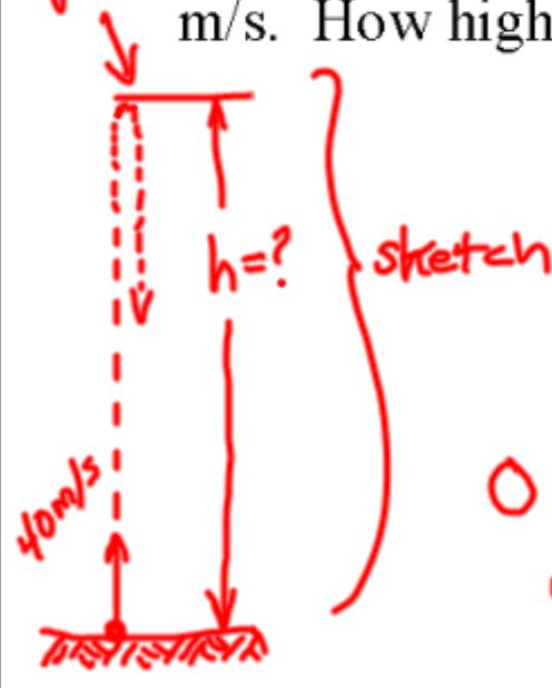
$$y = \frac{1}{2} a_y t^2 + v_{y0} t + y_0 \quad a = -g$$
