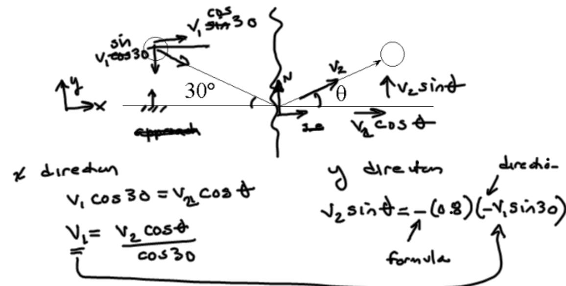
$$v_2 \sin \theta = 0.8 \frac{v_1 \cos \theta \sin 30}{\cos 30} = 0.8 v_1 \cos \theta \tan 30$$
