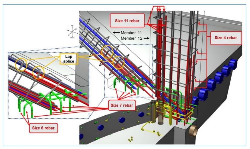
**Figure 17.** Main span, north end, showing rebar detailing in member 11, member 12, and node 11/12. Inset shows another view of rebar in node 11/12 and detail of lap splice from member 11. (Source: FHWA 2019)
