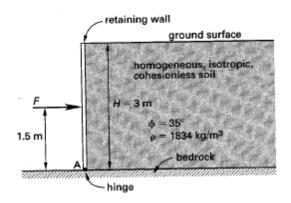
Using Rankine's theory, the total active resultant lateral earth force per unit length of retaining wall is most nearly
