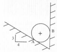
The wall reaction (N) at Point A is most nearly:
