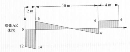
The maximum magnitude of the bending moment (kN•m) in the beam is most nearly:
