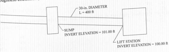
For full pipe flow with water surface elevations in the upstream sewer sump and lift station wet well of 105.00 and 103.50 ft, respectively, the discharge (cfs) is most nearly:
