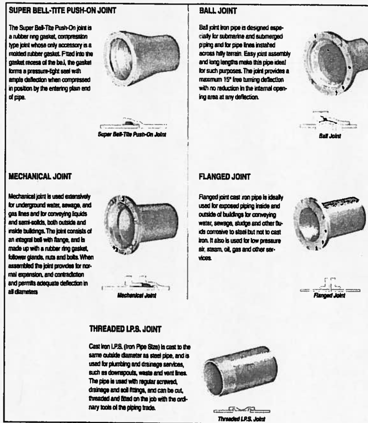
FIGURE 25.21 Joint connections for cast-iron pipe. (Reprinted with permission of McWane Cast Iron Pipe Company, Birmingham, AL)
