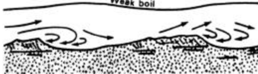
C. Dunes, surface waves out of phase with sand waves Boil
