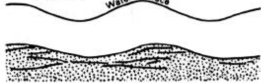
F. Antidune standing waves, surface waves in phase with sand waves Water surface
