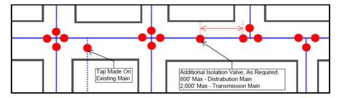
Isolation valves shall be placed on all fire hydrant leads. All fire hydrants shall have a mainline valve adjacent to the fire hydrant lead or positioned such that the closing of three valves shuts down the main and only puts one fire hydrant out of service.
