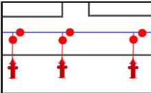
Isolation valves provided on both sides of the bore under State highways, railroads or large creeks/rivers.
