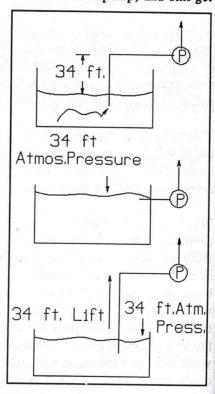
But how does this theoretical 34 ft. of water pressure (14.7 psia) become less than the theoretical vapor pressure of water (.59 ft., .256 psia)? It does happen, because these are both only theoretical, and static quantities.
