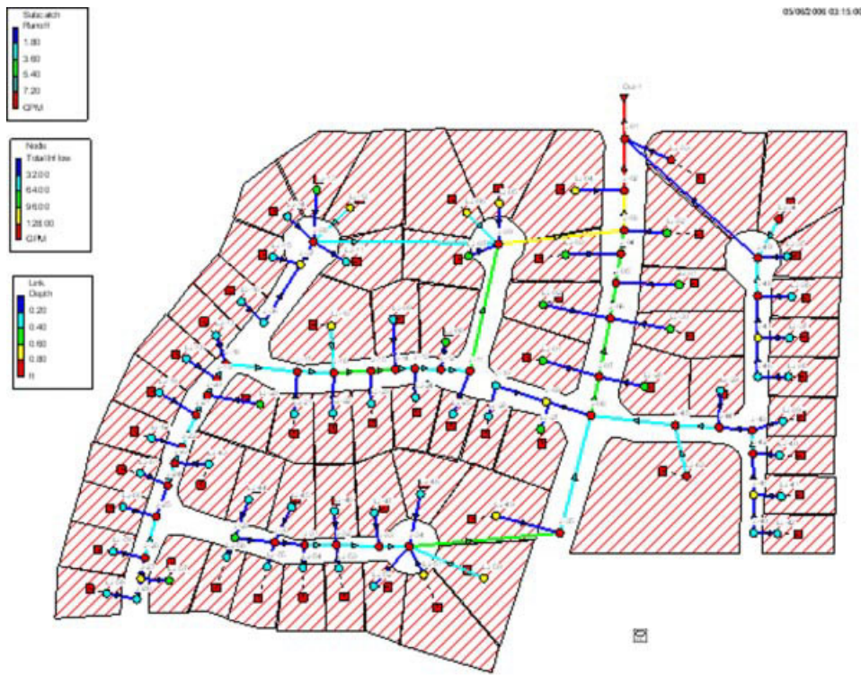
Figure 4 SWMM network at peak flow. [Color figure can be viewed in the online issue, which is available at www.interscience.wiley.com .]
