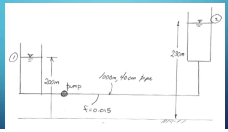
$$H_p = (30) + H_{\text{Loss}} = 30 + (f\frac{L}{D} + K_{\text{entrance}} + K_{\text{bend}} + K_{\text{exit}})\frac{Q^2}{A^2 2g} = 127Q^2 + 30$$
