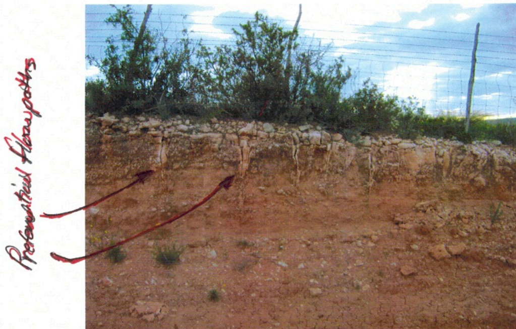
Figure 4.15. Photograph of a preferential flow feature in alluvium showing obvious signs of large-scale water intake over time. Photograph taken by the author, Tom Green County, Texas.
