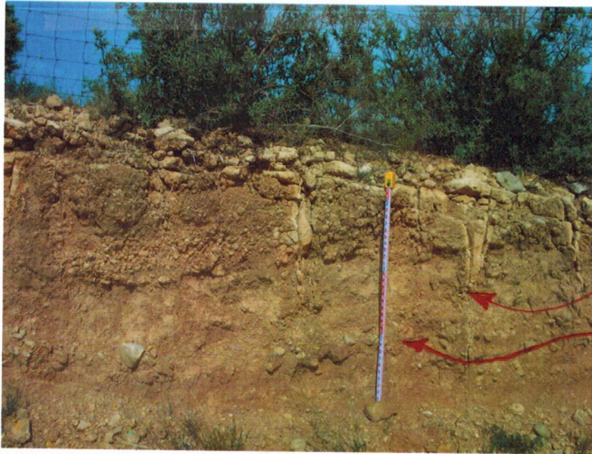
Figure 4.16. [Photograph of a preferential flow feature in alluvium showing obvious signs of large-scale water intake over time, Tom Green County, Texas.
