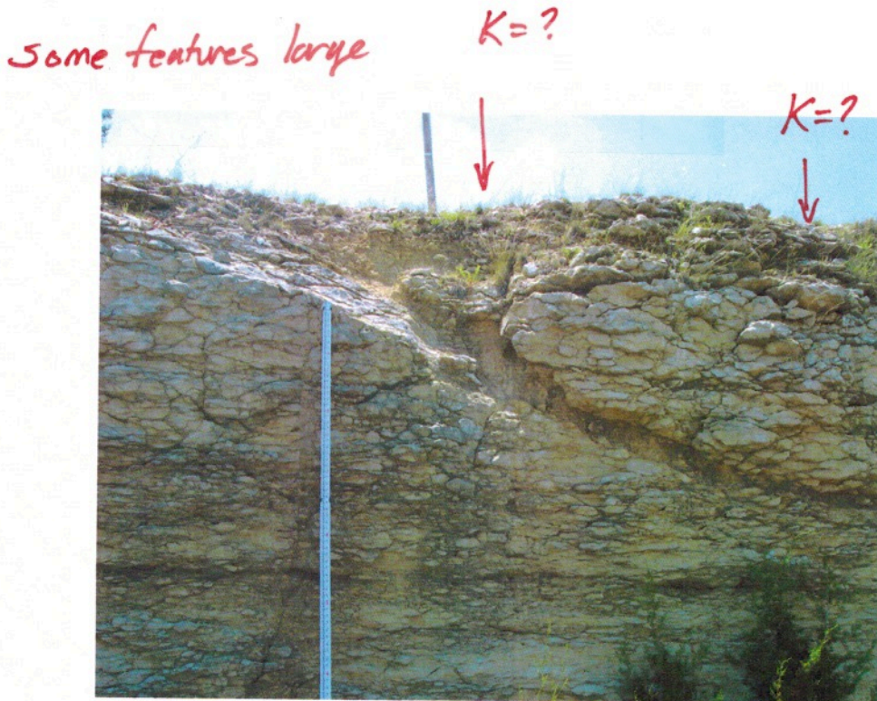
Figure 4.13. Photograph of feature in limestone showing obvious signs of large-scale water intake. Photograph taken by the author on US 277 in Schleicher County, Texas.
