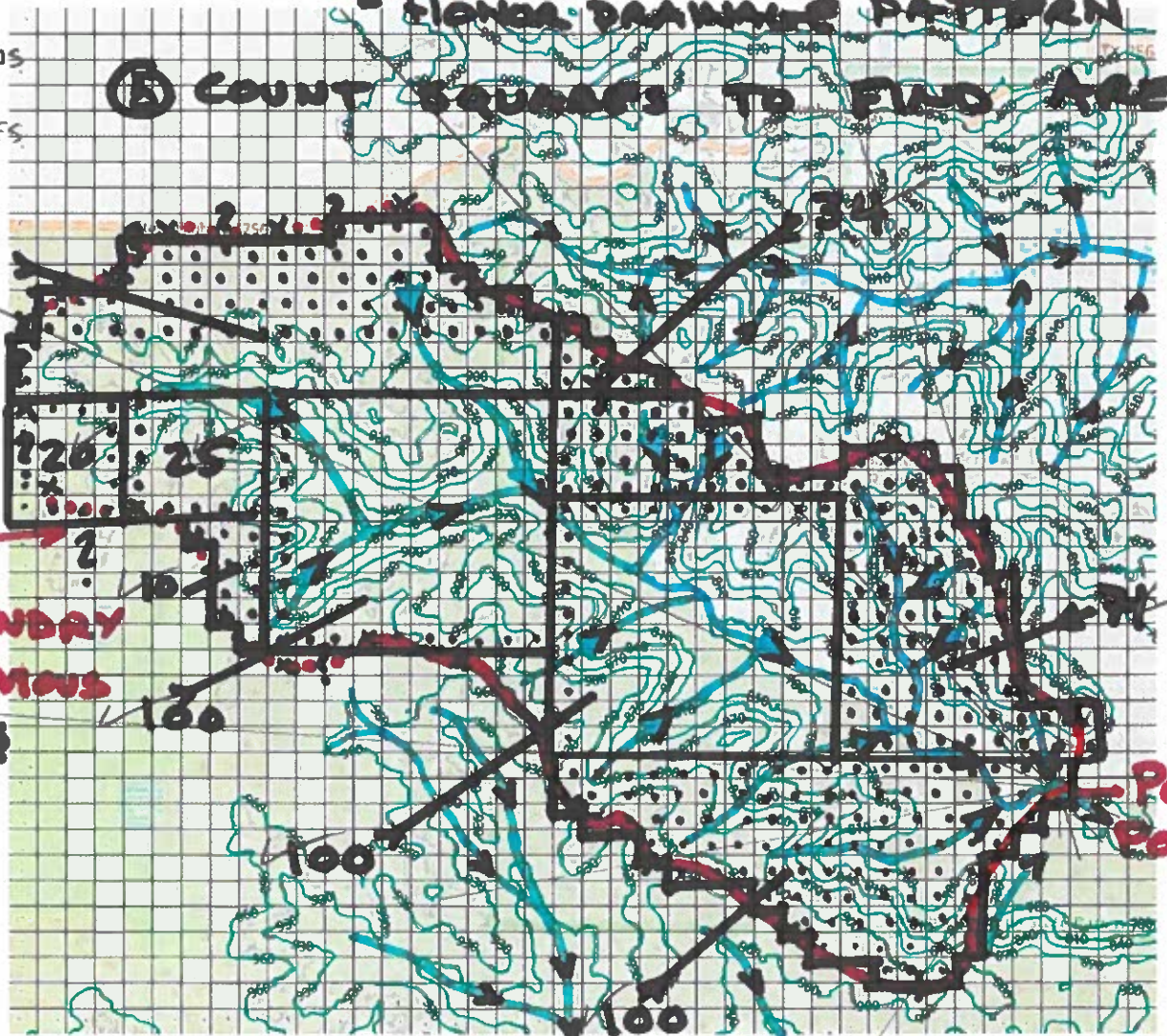
Figure 4: Topographic Map of a portion of the Earth. Elevations are in meters. Each square is 150 meters on a side. North (by convention) is up.
