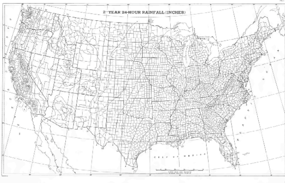
Figure 3: Selected map from TP-40. The map depicts the United States with contour lines of estimated rainfall depth (isohehets) for the specified probability and duration. Several such maps are in the report, along with methodology and interpolation procedures to infer values not mapped.
