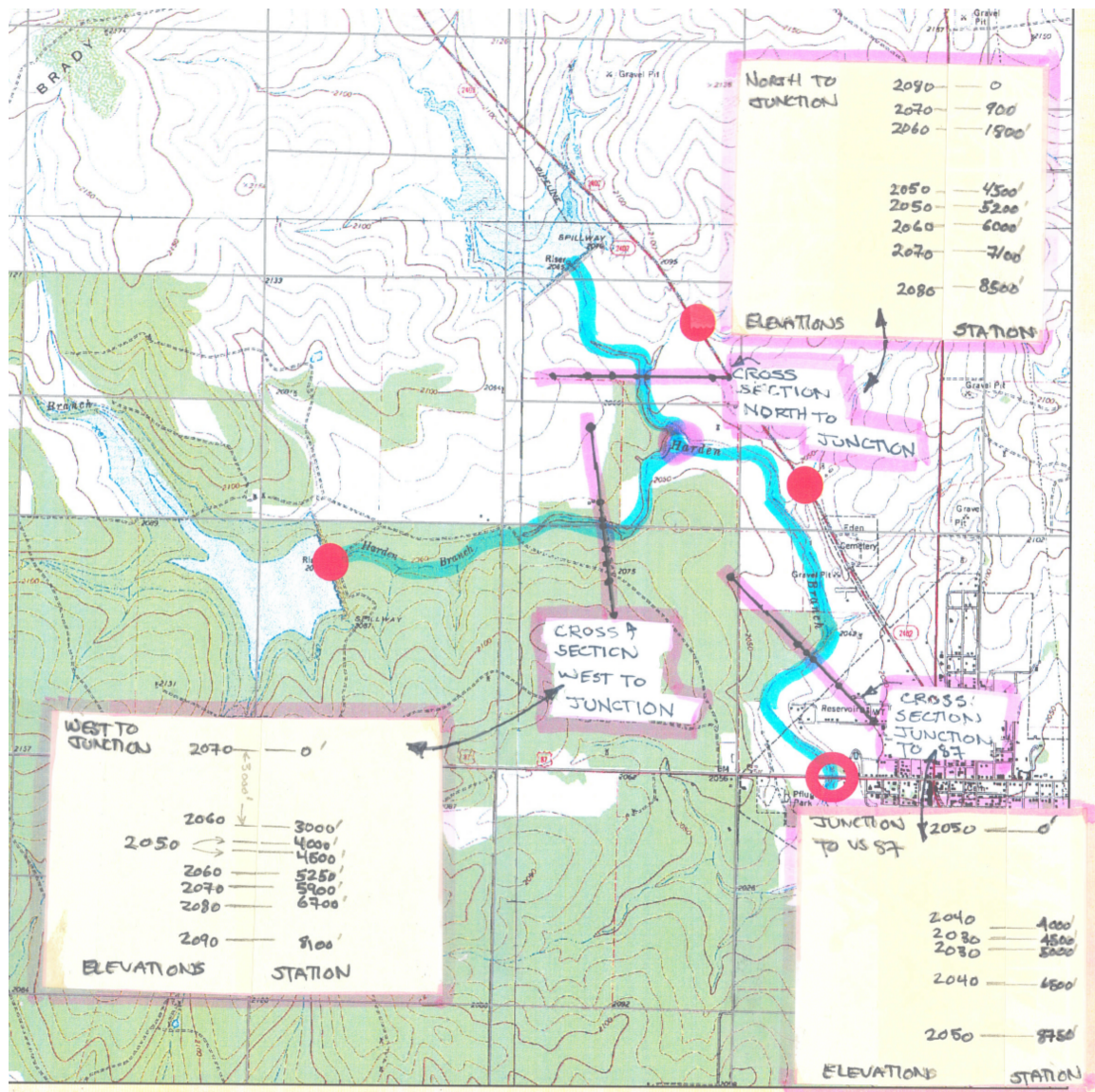
Figure 24. Cross section locations used to approximate channel geometry for Muskingum-Cunge routing in HEC-HMS
