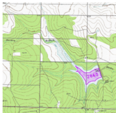
Figure 3: Reservoir impounds water, but outlet works inactive because water is not deep enough yet. Approximate 2070 foot pool area shown (mislabeled as 2060)
