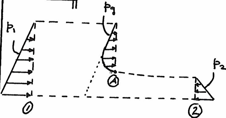
PRESSURE AT GATE (A) IS NOT HYDROSTATIC - NEED A DIFFERENT APPROACH
