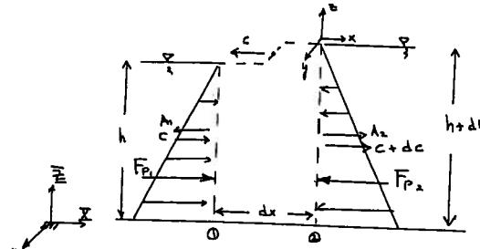
Steady flow, moving C.V.
