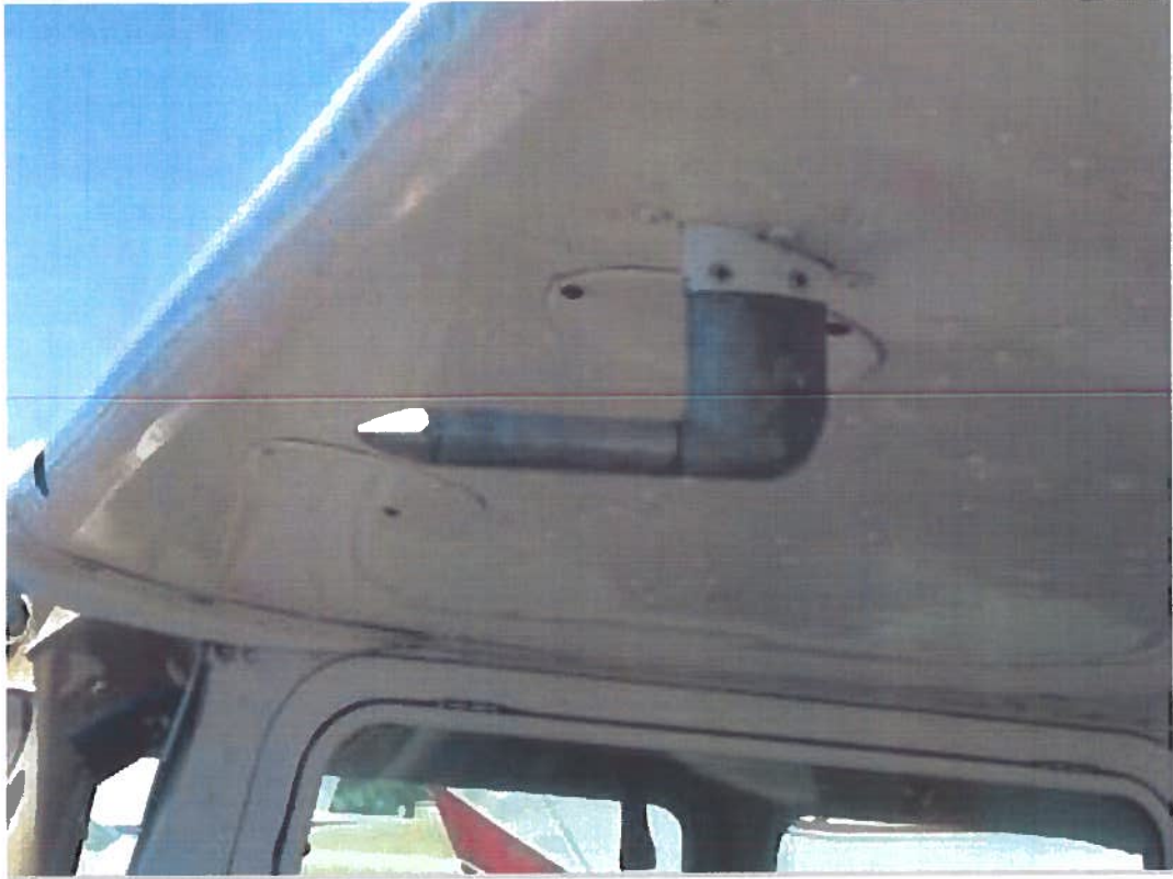
PITOT-STATIC TUBE ON LIGHT AIRCRAFT
