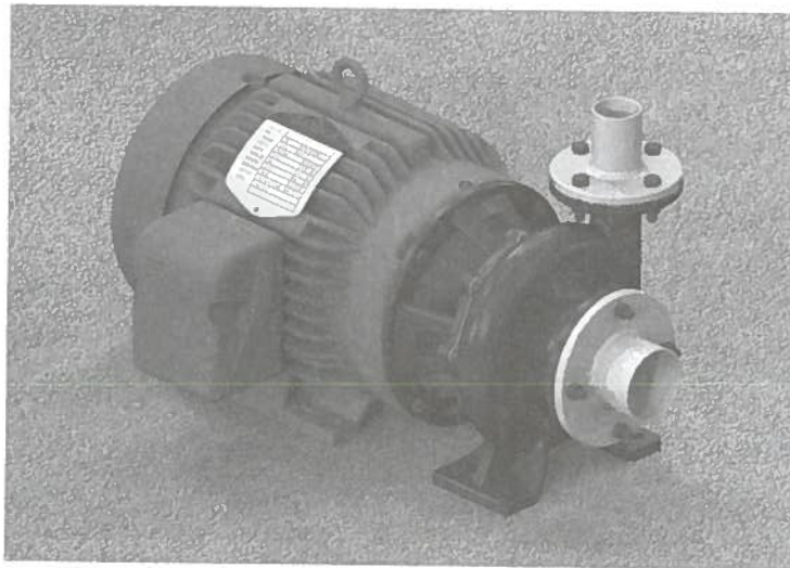
FIGURE 7.7 CAD drawing of a centrifugal pump and electric motor. (Image courtesy of Ted Kyte; www.ted-kyte.com .)
