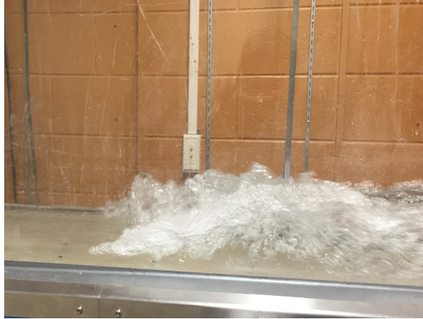
Figure 2: Hydraulic Jump in the Laboratory Experiment
