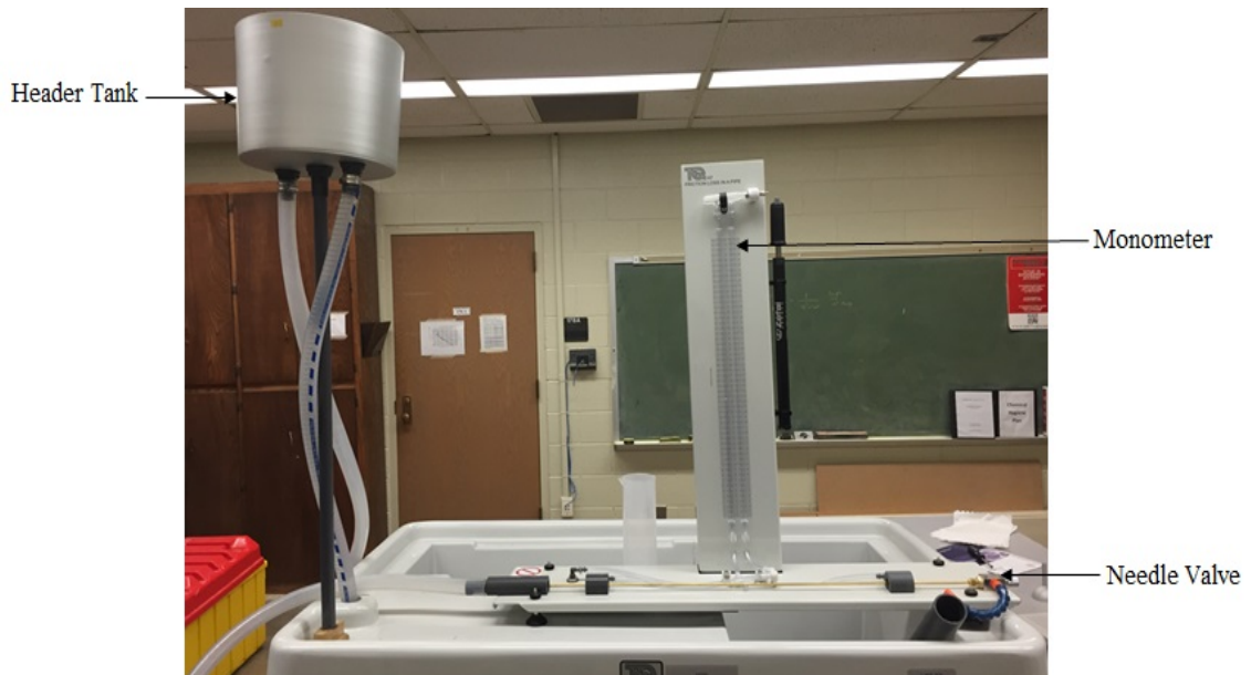
Figure 1: Experimental Setup of Friction Loss in a Pipe
