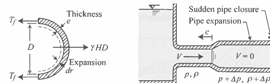
Figure 6.2 Wave propagation in an elastic pipe
