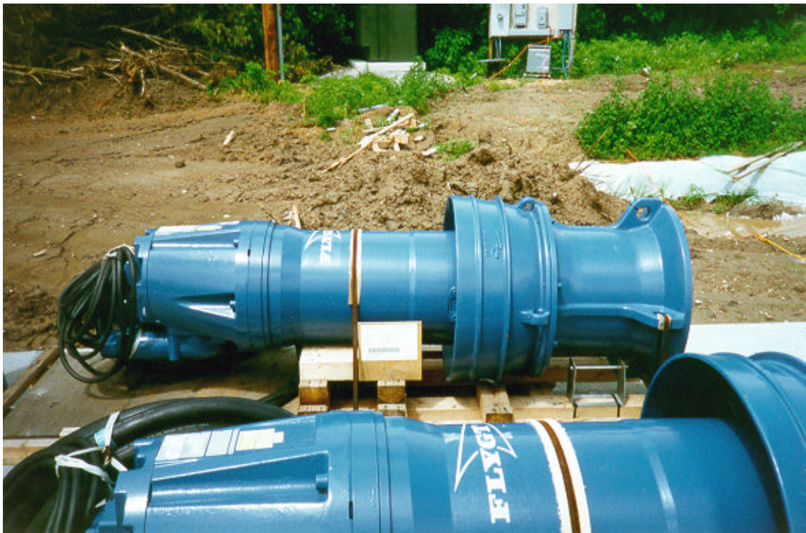
Figure 3-11. Large submersible pumps
