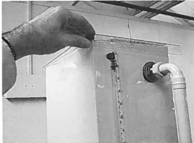
Figure 14 Fit the Lid to the Reservoir
