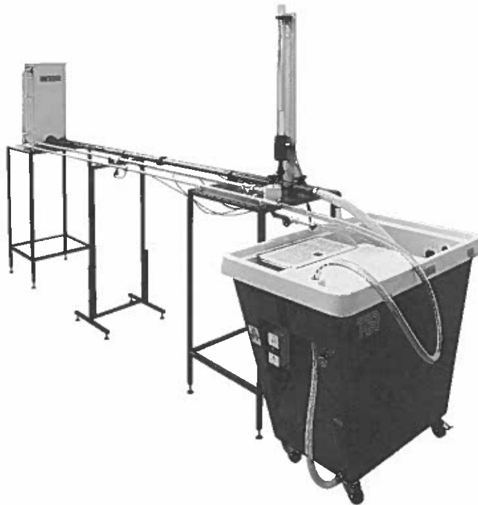
Figure 1 H405 Pipe Surge and Water Hammer
