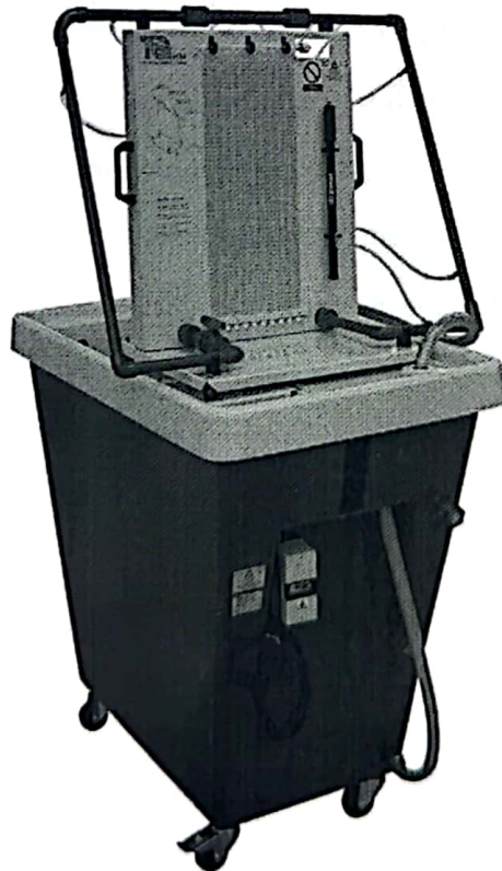
Figure 4 The H34 on Top of a H1d Hydraulic Bench
