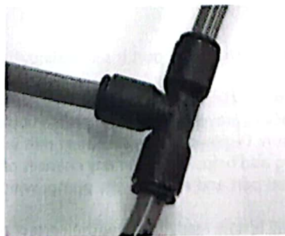
Figure 2 You May Cut Existing Pipes and Fit a 'T' Piece (not supplied)
