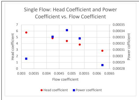
**Figure W: Single Flow Dimensionless Characteristics.** Note the multiple axes.
