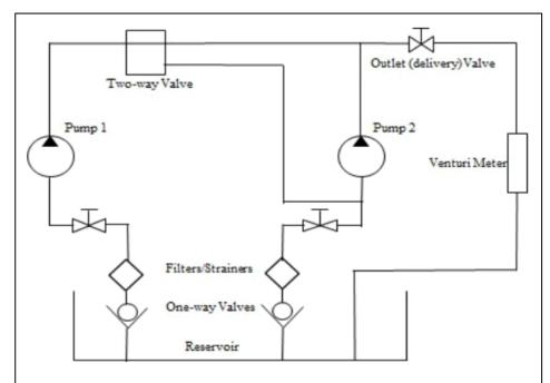
**Figure 1: Fluid Pathways Provided by Experimental Machine.**Note that the different paths allow for 3 different types of flow: single, parallel, and series.
