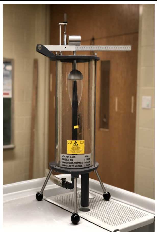
Figure 4. Hemispherical Cup Vane Apparatus. This setup was used for the second portion of the experiment.
