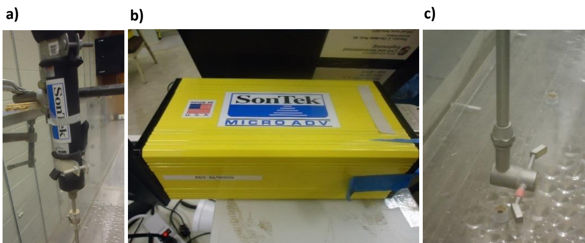
Figure 4.6 - Different components of the used ADV: a) conditioning module; b) processor; c) 2D side-looking probe.
