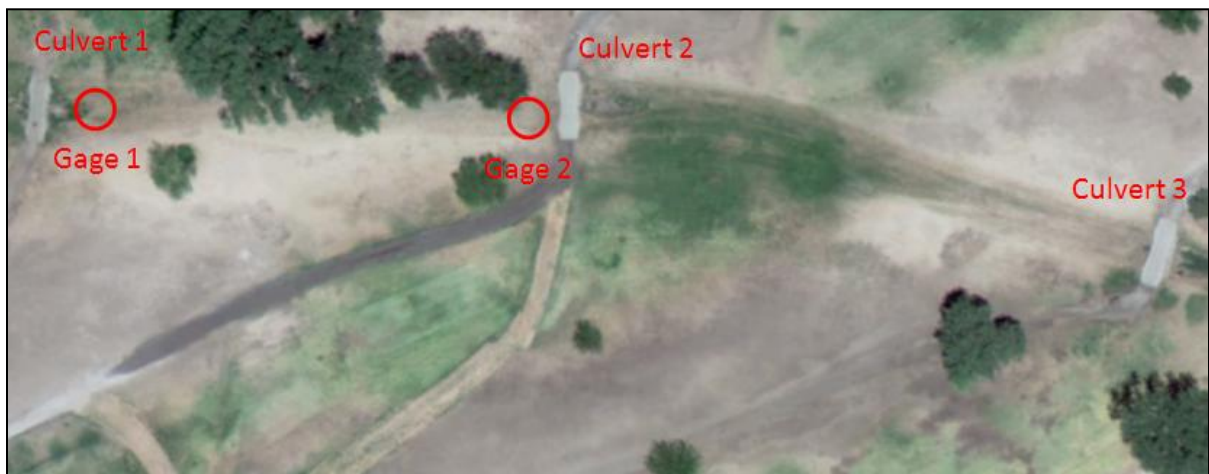
Figure #. Satellite imagery of the culvert paths and the USGS crest-stage gages at the John Pitman Municipal Golf Course.
