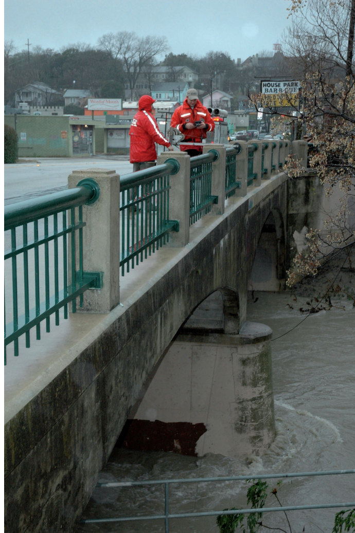
Figure A.1. U.S. Geological Survey (USGS) personnel conducting one of two high-magnitude discharge measurements on January 11, 2007 at USGS streamflow-gaging station 08156800 Shoal Creek at West 12th Street, Austin, Texas. Both measurements are represented in the database used for this paper. Photograph by W.H. Asquith and courtesy of USGS.
