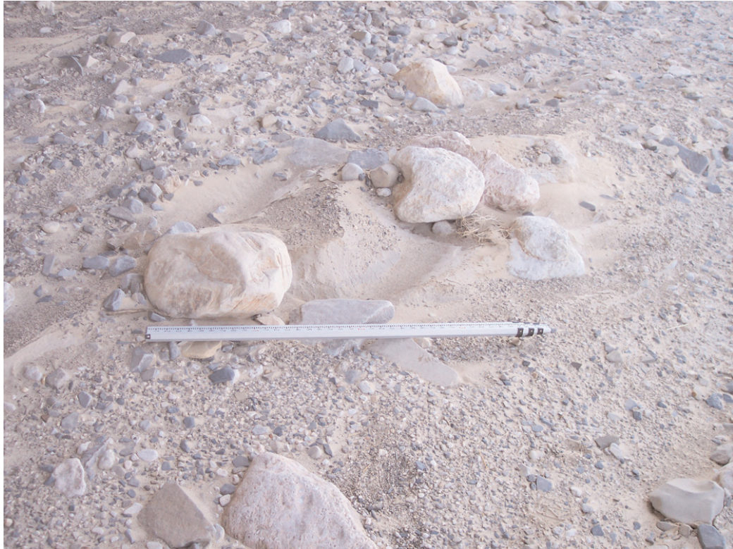
Figure 2.5. Large bed material (4 ft. Philadelphia level rod for scale).
