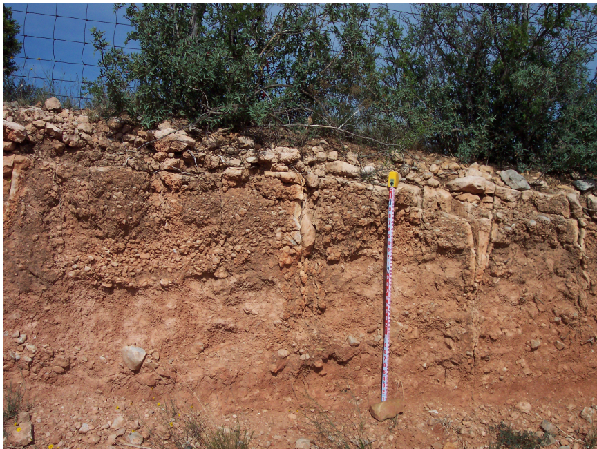
Figure 4.16. [Photograph of a preferential flow feature in alluvium showing obvious signs of large-scale water intake over time, Tom Green County, Texas.
