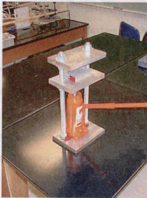
Figure 2-2 Example of an apparatus used for fabrication of MEA's.
