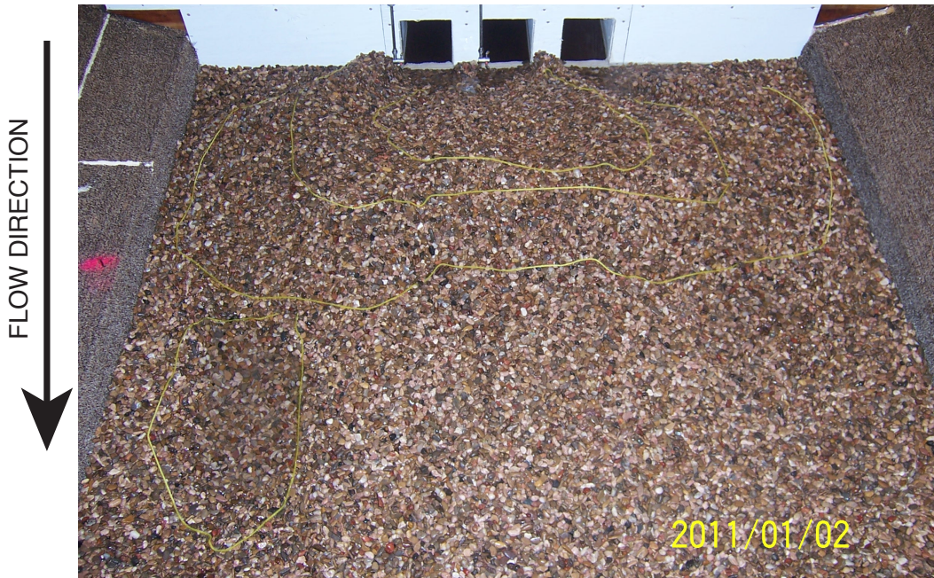
Figure 3.26. Photograph of Downstream Bedform Following Experiment on 2011/07/22, Experimental Model M-R
