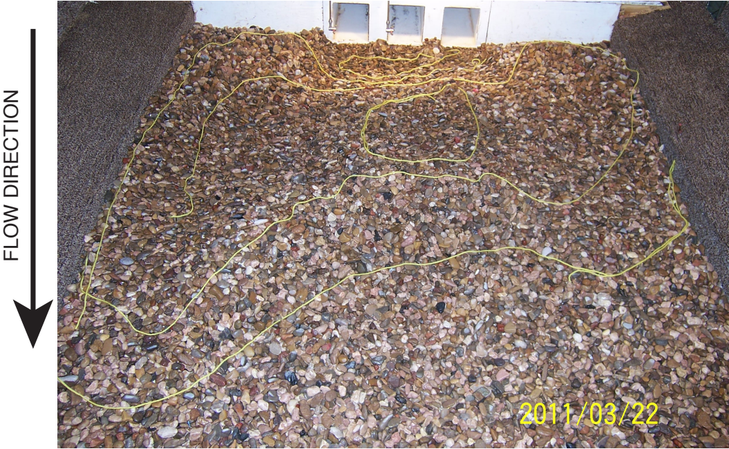
Figure 3.19. Photograph of Downstream Bedform Following Experiment on 2011/03/22, Experimental Model M-R
