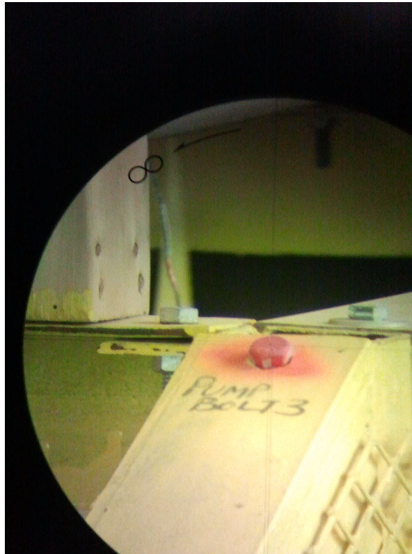
Figure 3.14. Benchmark pumpbolt3 as Seen Through the Eyepiece of the Total Station
