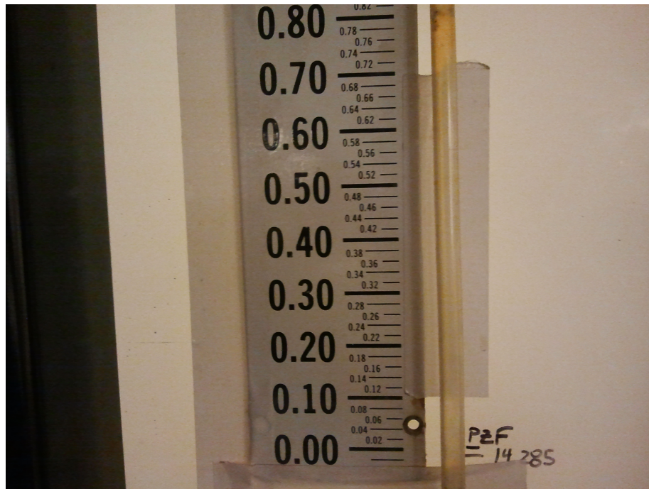
Figure 3.10. Sight Glass Used to Measure Head in the Head Tank
