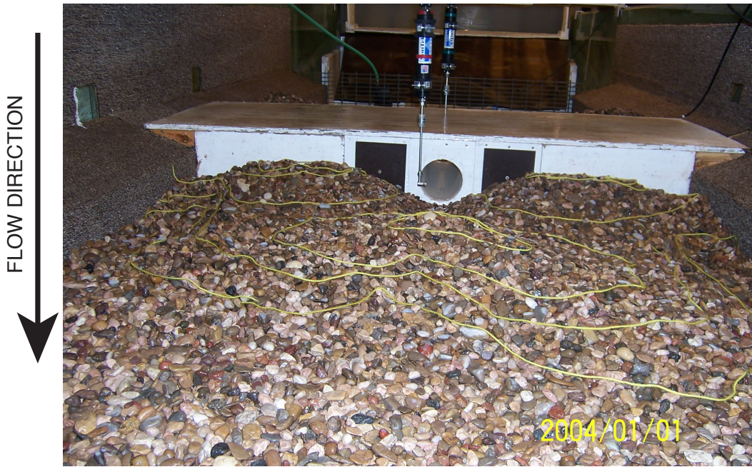
Figure 3.22. Photograph of Downstream Bedform Following Experiment on 2011/04/01, Experimental Model S-6-C
