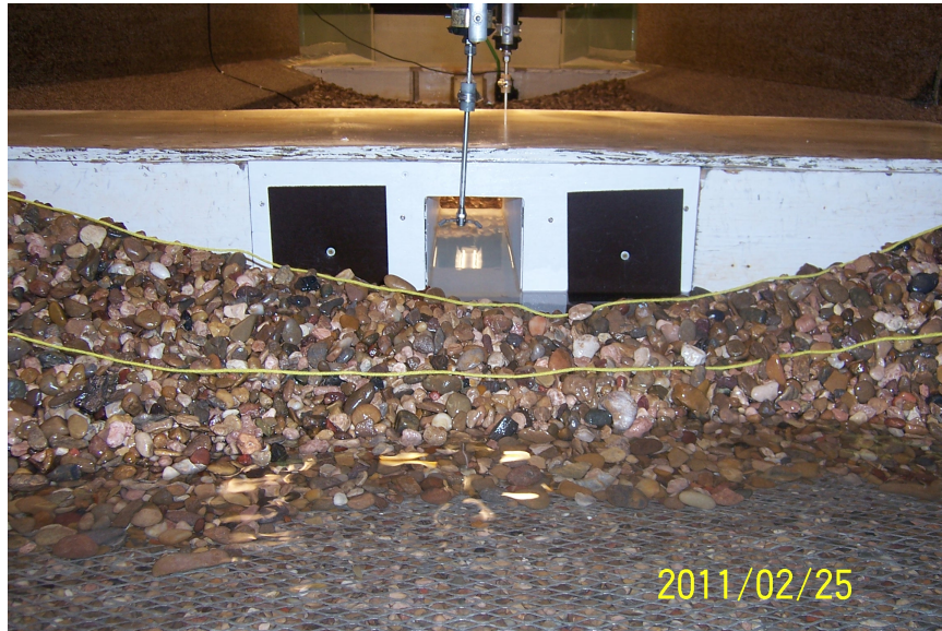
Figure 8.15. An example on how the sediment dune eroded in the center as transportation continued through the culvert.
