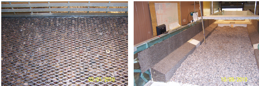
(a) Picture of the aluminum screen trapping the lowest layer of sediment particles. (b) Outdoor carpet applied to stream banks and glass walls.
