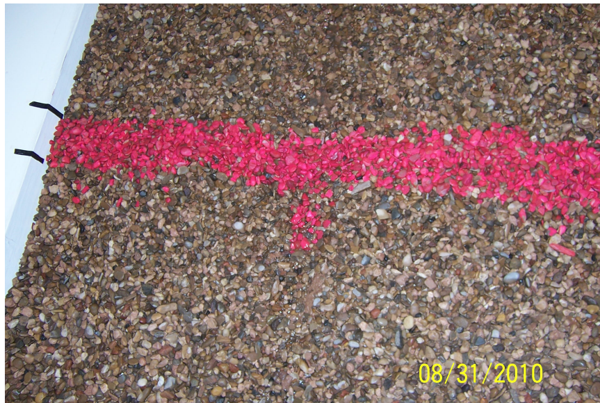
Figure 4.2. Sediment trial movement showing no movement to the pink rocks.
