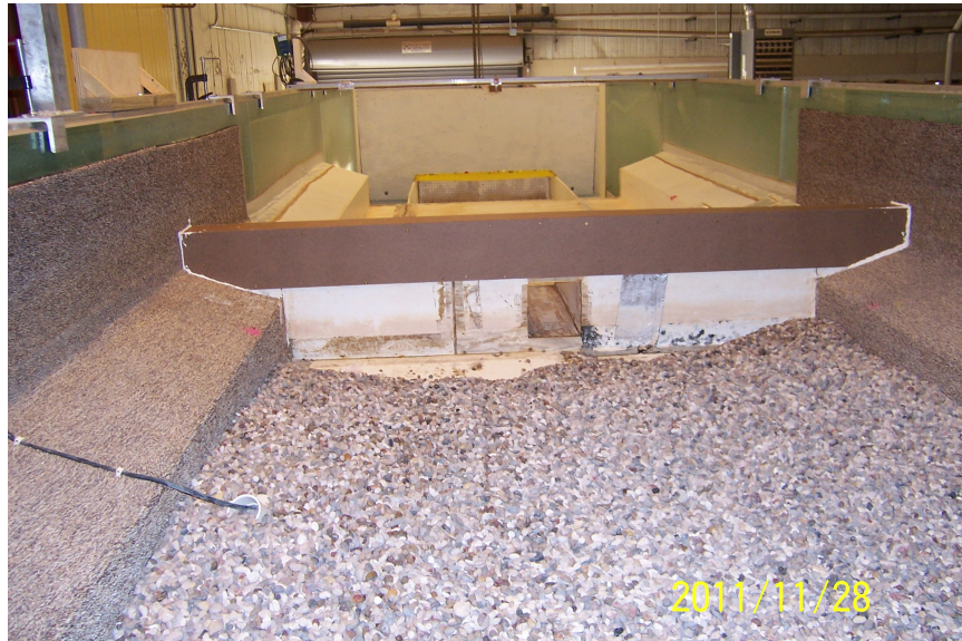
Figure 8.23. A picture showing the downstream control's road raised in height
