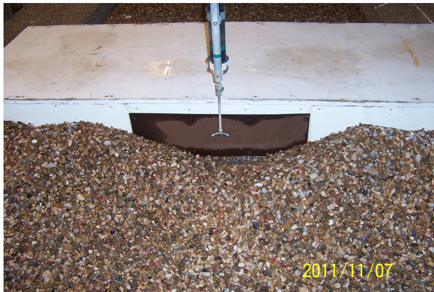
Figure 8.4. Cavity in sediment bed developed by the flow patterns in the channel
