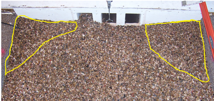
Figure 4.4. Sediment placed in the corners of the stream channel
