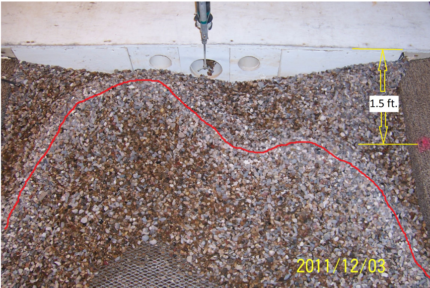
Figure 8.25. Sediment dune position with larger depths
