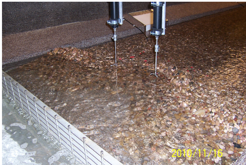
Figure 5.1. MicroADV's tracking the sediment dune migration
