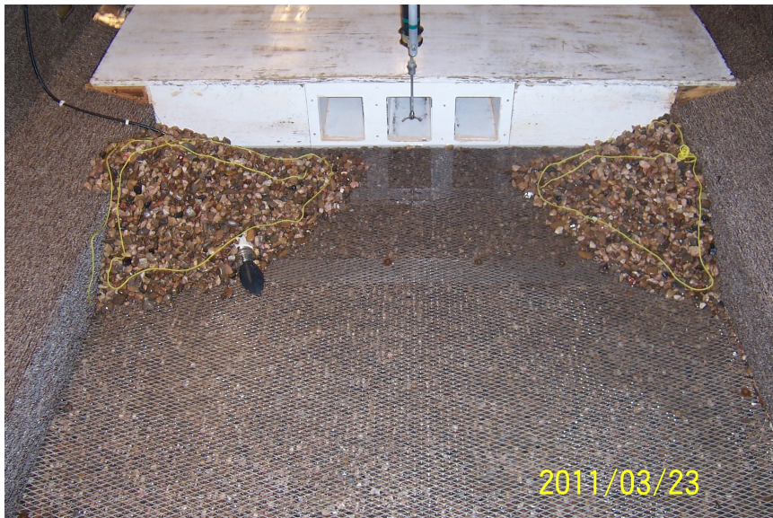
Figure 8.13. Large sediment movement leaving the floor exposed
