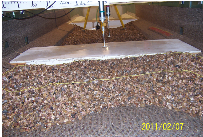
Figure 8.2. A photograph showing the sediment dunes height in reference to the road deck
