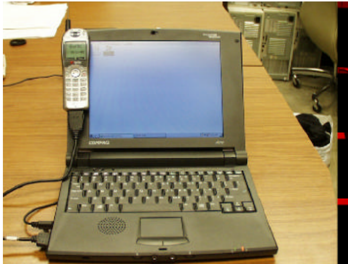
Figure 67. Hardware/Software for PDA/Cellular connection (Compaq Aero 8000)
