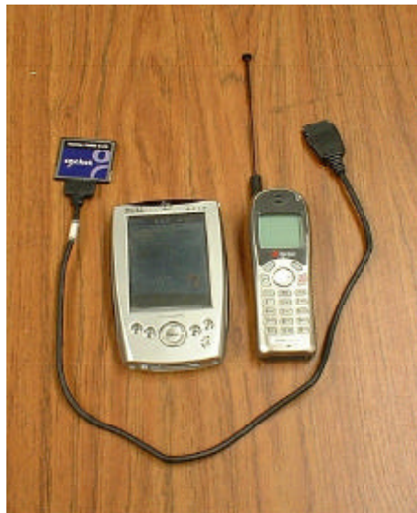
Figure 38. Hardware/Software for PDA/Cellular connection (Dell Axim PDA)
