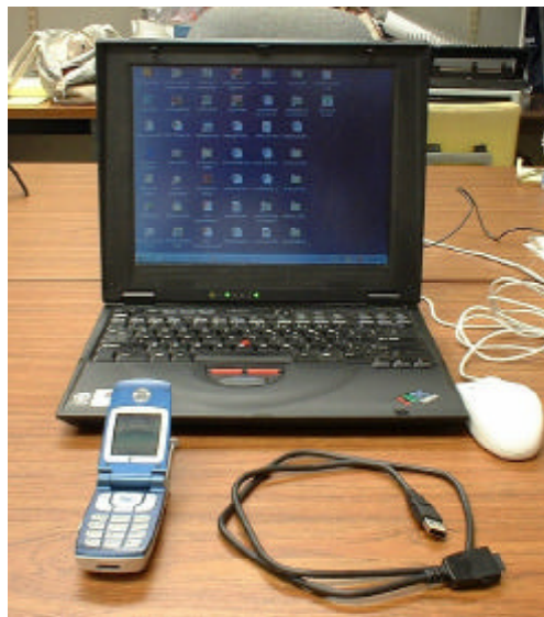
Figure 24. Hardware/Software for Laptop/Cellular connection (IBM Laptop PC)
