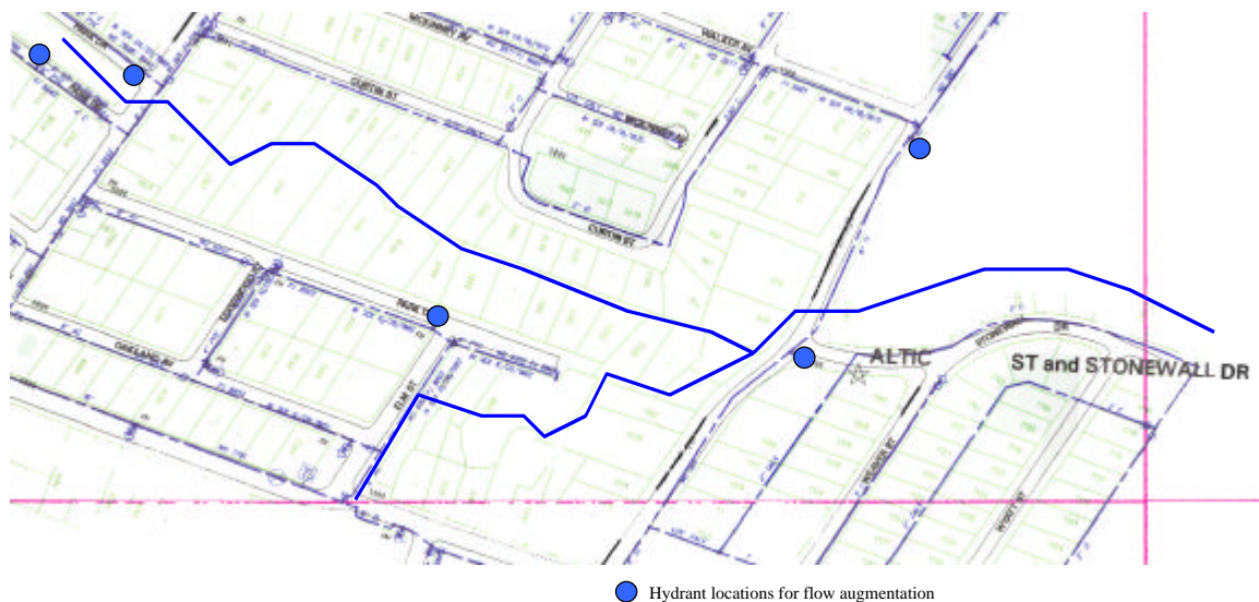
Figure 7.1 GIMS map of possible hydrant locations for flow augmentation. (Blue lines are approximate alignment of Bayou)
